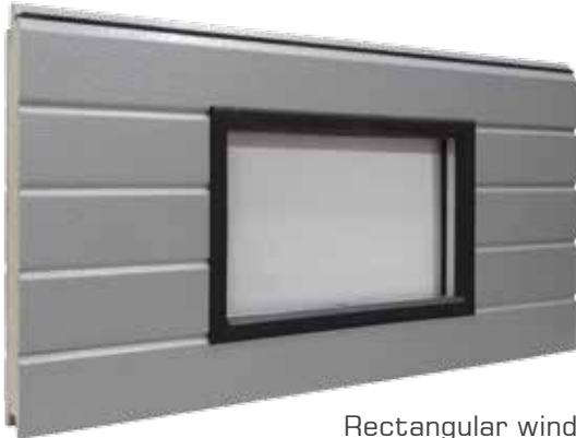
Rectangular window Black plastic frame Double acrylic glazing Dimensions — 488x322mm
