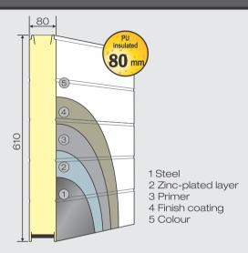
Ultra Thermo Industrial door is designed and manufactured to save Thermal energy in heated or refrigerated premises. The thermo brake between inner and outer steel surfaces and 80 mm thick, high density polyurethane insulation provides excellent thermal value of the door up to 0.5 W/m² K.
